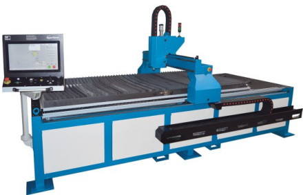
Machine control and operation are done on the main control panel which is located in front of the machine
