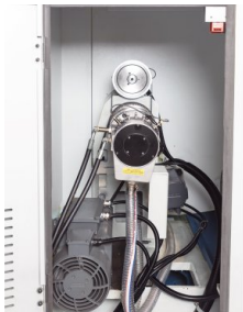
48 mm spindle bore in draw-tube
