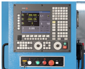
Compact control unit with electronic hand-wheels
